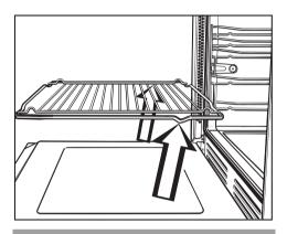
When pushing the tray, pan and rack back in, always ensure that the safety notches are at the rear of the oven. (See illustration).
